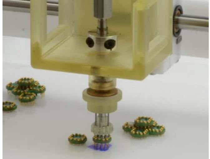
Fig. 13 The Bitblox printer’s toolhead, which uses pin-in-socket connections to manipulate the material blocks.
