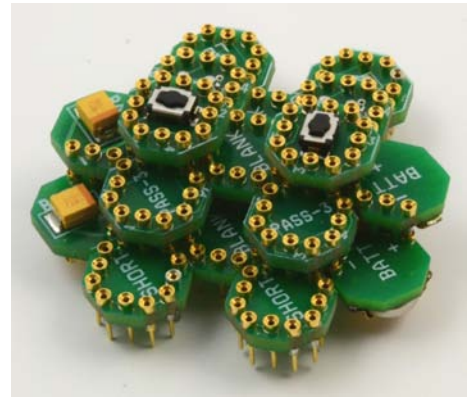
Fig. 14 Two channels (play and stop) of an infra-red remote control printed with the Bitblox printer.
